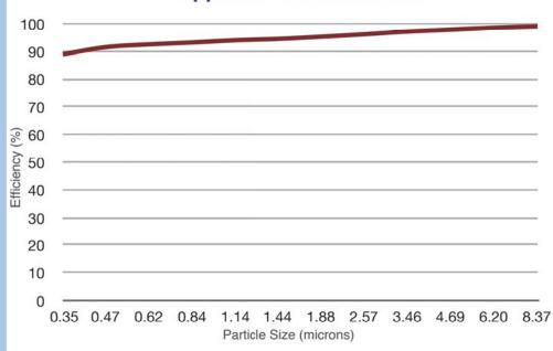
Tri-Dim's ULTRA Xe achieves a MERV 15 efficiency when tested under Appendix J of ASHRAE 52.2-2007.
