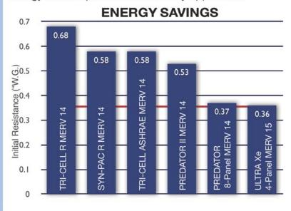
In a recent study that compared Tri-Dim's ULTRA media to conventional micro-glass filtration media, actual energy savings of 40% were documented by using precise equipment to monitor actual energy usage - not one of the many energy saving formulas or calculators.
